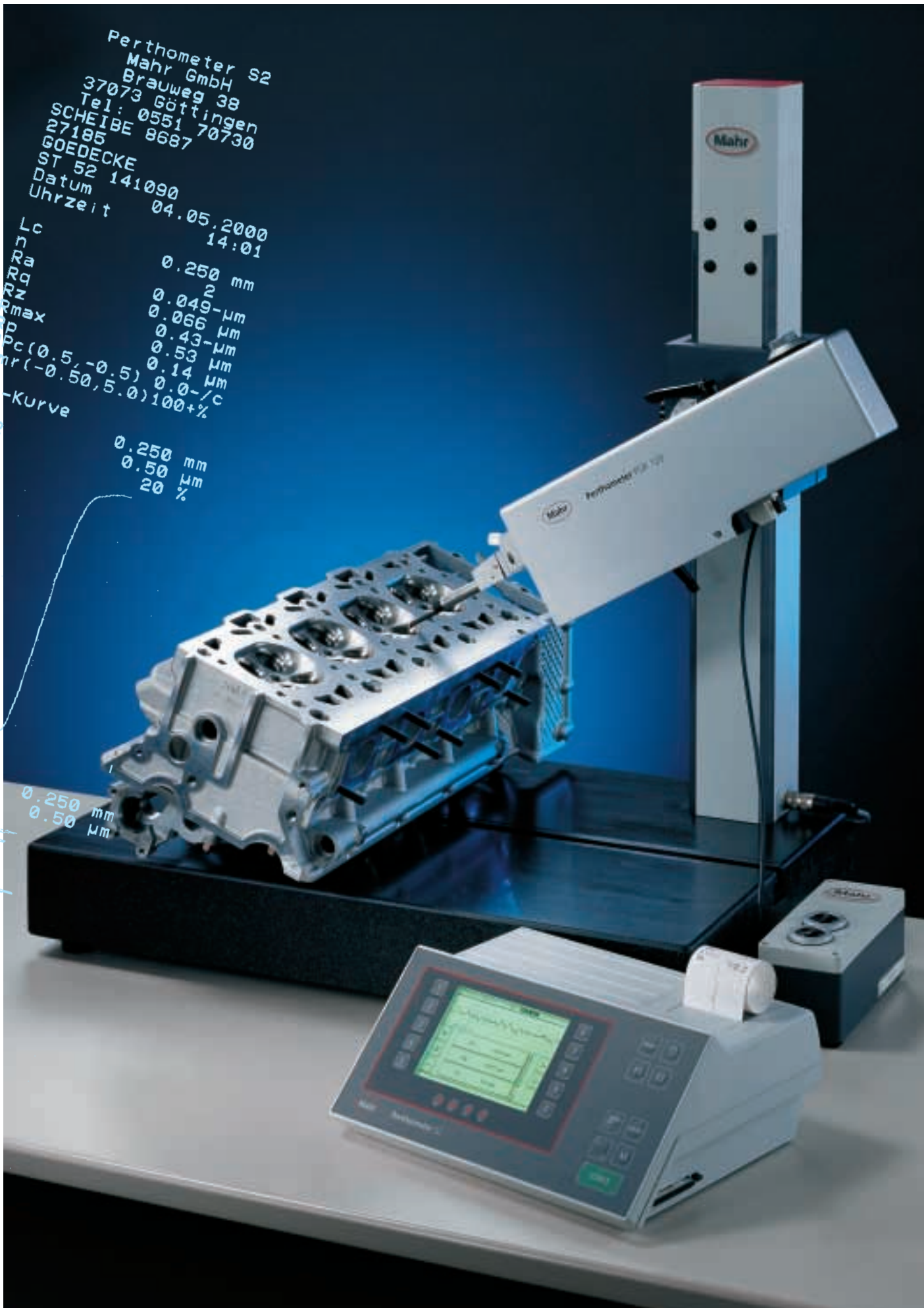
Perthometer S2 with PGK 120 and swivel device on measuring stand
