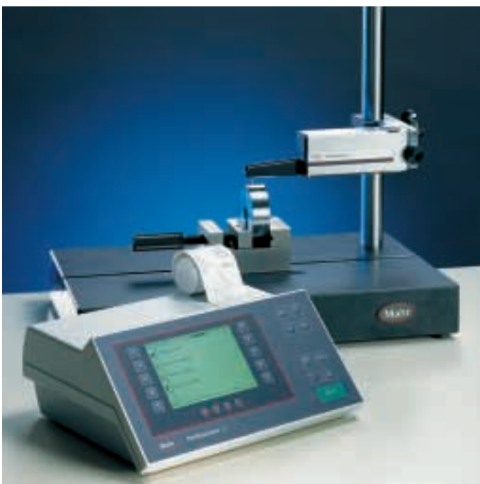
Perthometer S2 with PGK 120 and PST-G measuring stand
