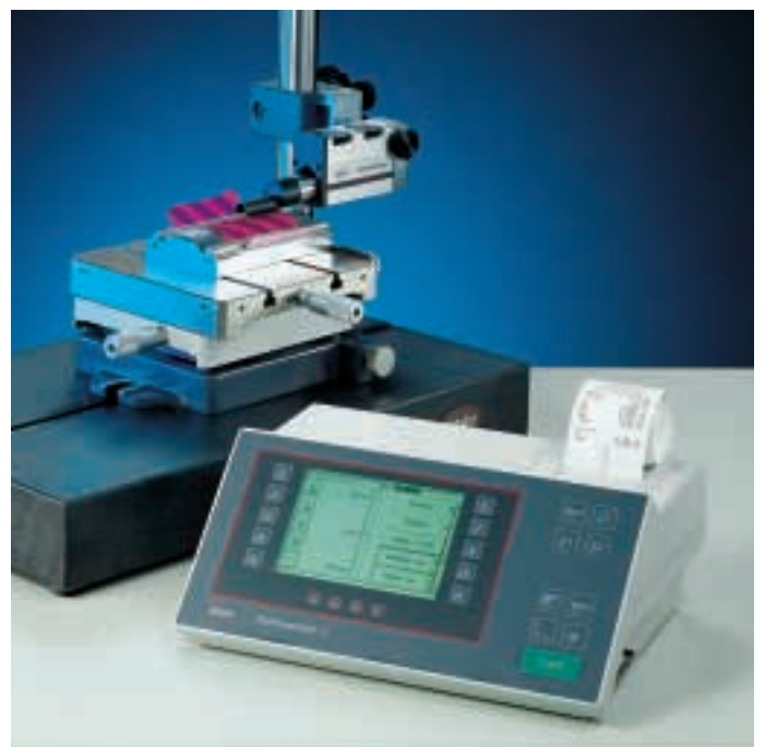
Foil measurement with Perthometer S2 and PZK
